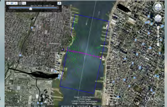
Hudson River RiverSonde radial velocity vector map (green) with cross-channel velocity profile in magenta.
