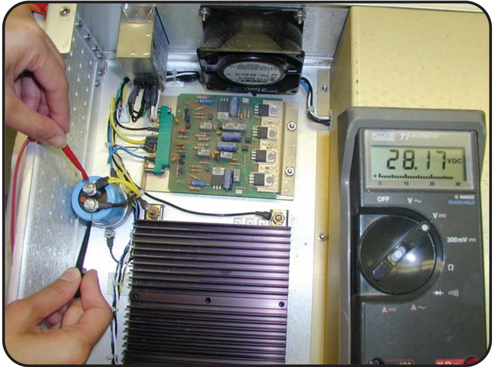
Measuring the Vicor 28 VDC Power Supply
